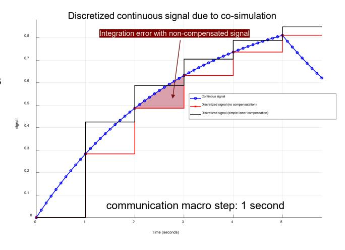
The compensated signal (black line) with simple linear extrapolation is closer to the ideal, continuous signal (blue line) than the uncompensated, discretized signal (red line)
