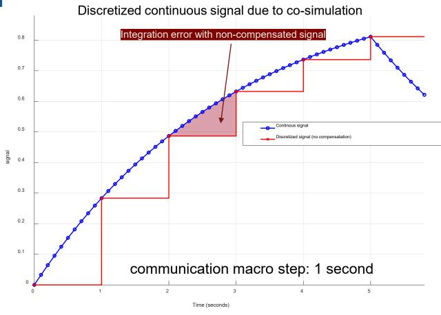
The un-compensated signal (red line) deviates from the ideal, continuous signal (blue line) due to discretization
