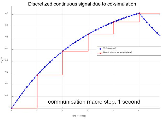
The un-compensated signal (red line) deviates from the ideal, continuous signal (blue line) due to discretization
