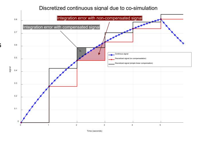
The compensated signal (black line) with simple linear extrapolation is closer to the ideal, continuous signal (blue line) than the uncompensated, discretized signal (red line)
