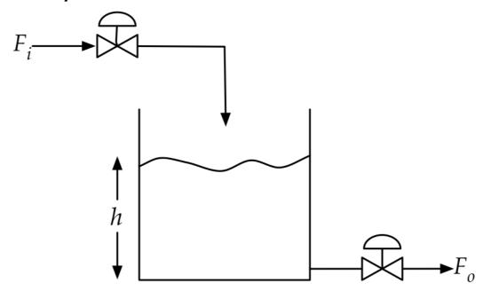
**Goal:** Control liquid level h(t) (CV) by adjusting inlet flow  $F_i(t)$  (MV)
