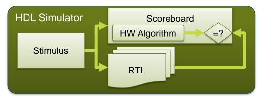
Generate SystemVerilog DPI/UVM verification test bench components
