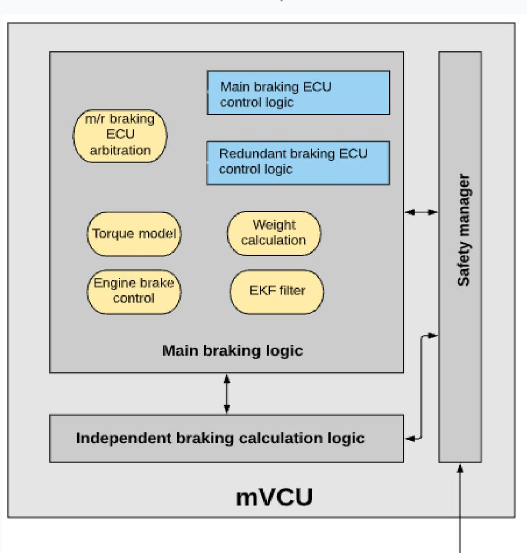
Solution: VCU software has symmetric design with both main braking logic and safety monitoring logic in each VCU.
