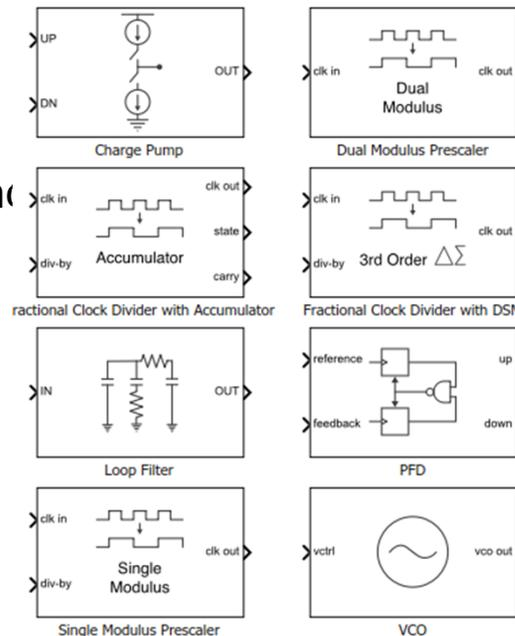
**Block Parameters: Fractional N PLL with Delta Sigma Modulator**
