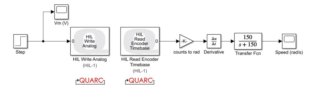
The virtual twin of the Quanser QUBE contains a servo motor and an inertia disk
