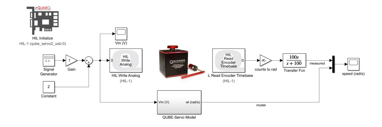
When on-campus, HiL write and read calls are executed via a USB interface against the real twin
