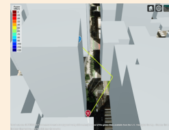
Manipulate phase of reflected rays by changing the material
