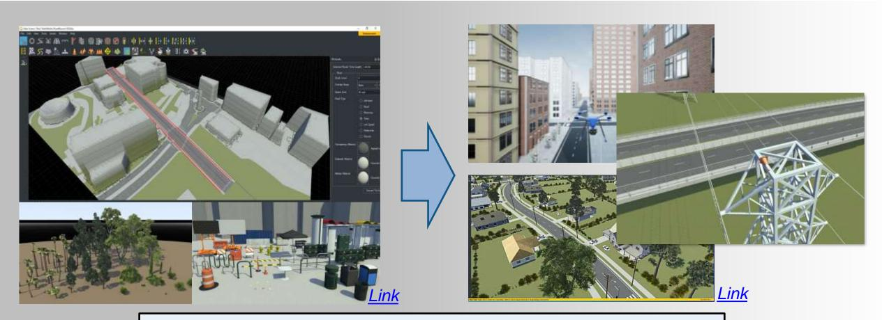
Design 3D scenes for simulating and testing autonomous algorithms
