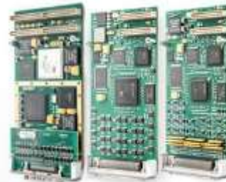
I/O modules installed in target machine
