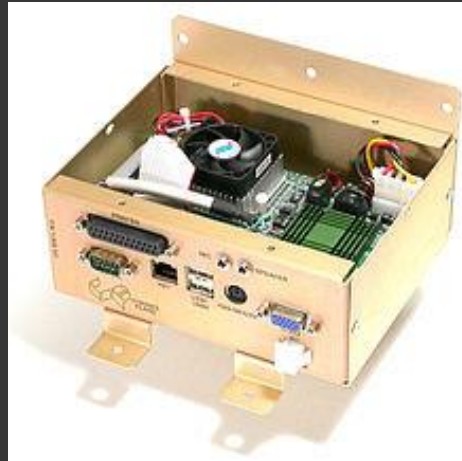
Embedded Computer Sub-Assembly for Accupoll Electronic Voting Machine
