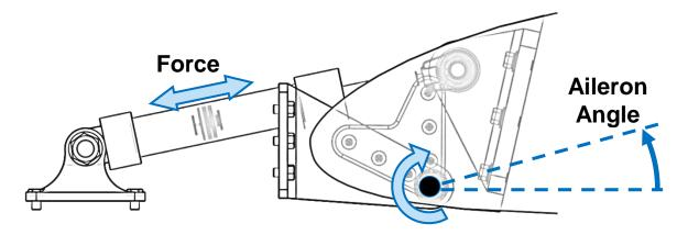
**Problem:** Determine the requirements for an aircraft aileron actuator
