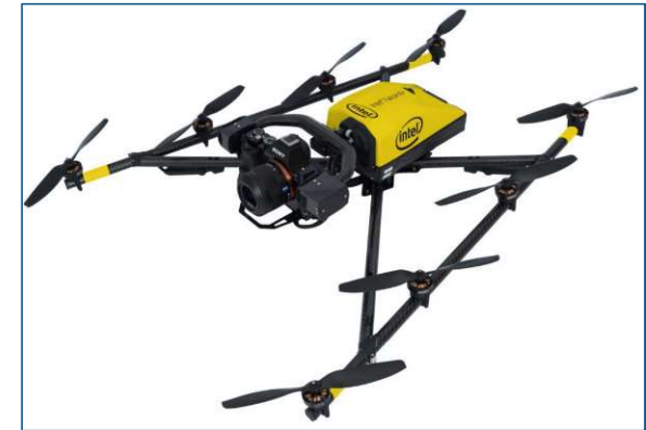
The eight-rotor Intel® Falcon™ 8+.
