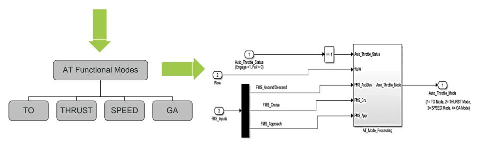
Note: The flow charts are the model representation for high level textual requirements. The simulink models are representation of lower lever requirement derived from the high level requirements model
