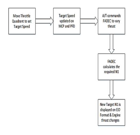
**AT Engagement/Disengagement:** Push button located on TQA. To prevent inadvertent thrust at time of disengagement, throttles will be moved to position consistent with current supplied thrust. Pilot can override this movement by moving the throttle manually
