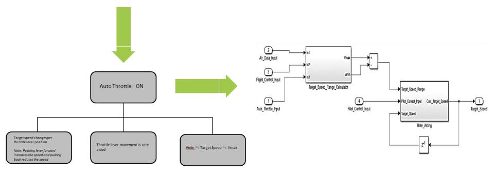
Note: The flow charts are the model representation for high level textual requirements. The simulink models are representation of lower lever requirement derived from the high level requirement model
