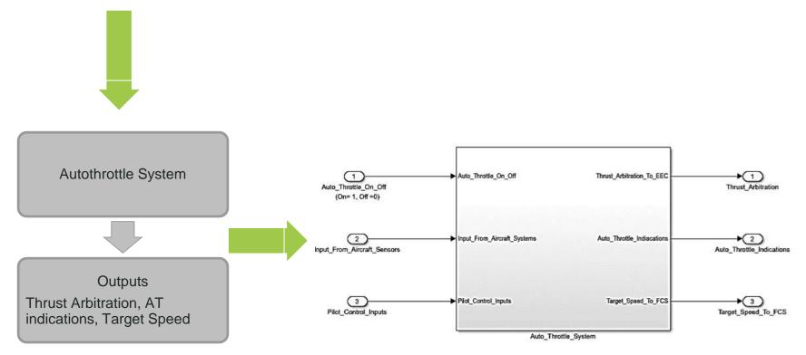
Note: The flow charts are the model representation for high level textual requirements. The Simulink models are representation of lower lever requirement derived from the high level requirement model
