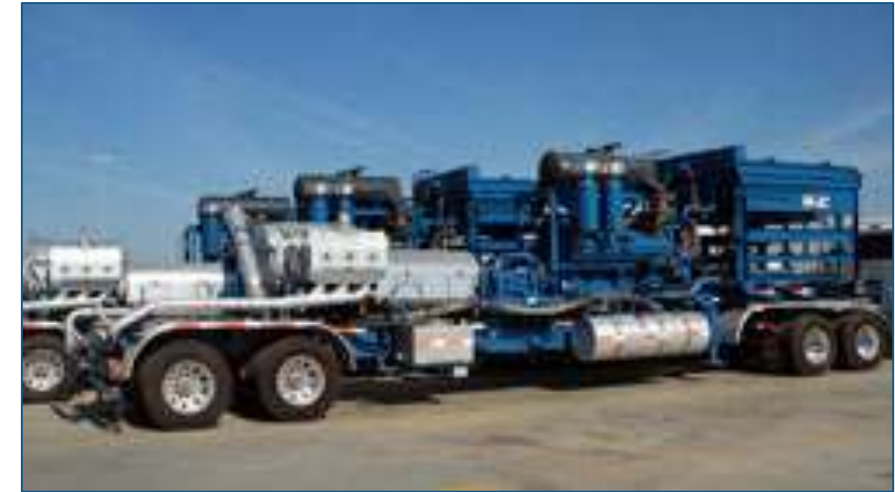
Truck with positive displacement pump.
