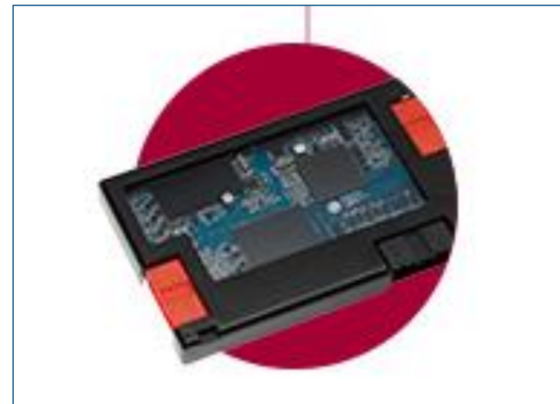
The LG Chem battery management system.
