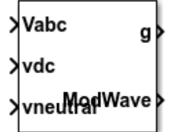
PWM Generator (3-phase, 3-level)
