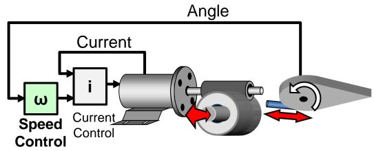
**Problem:** Optimise the speed controller to meet system requirements
