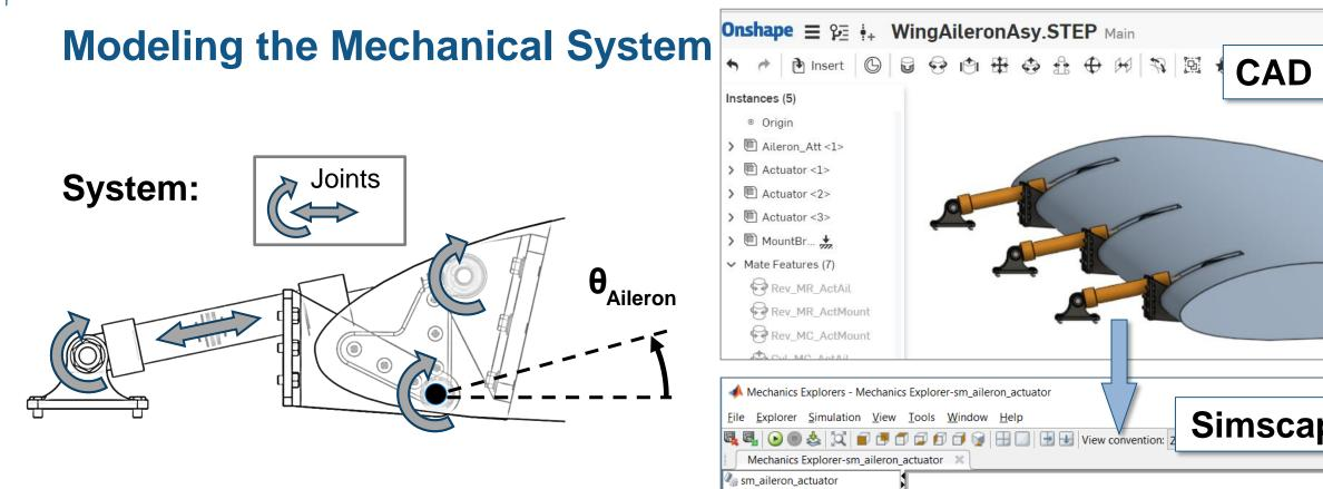
**Problem:** Model the mechanical system within Simulink
