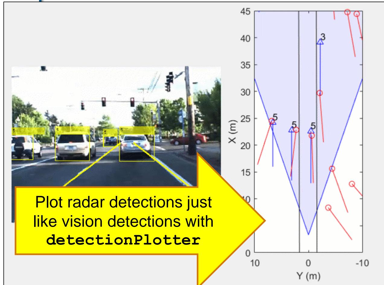
Plot radar detections just like vision detections with **detectionPlotter**
