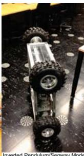
Inverted Pendulum/Segway Mode
