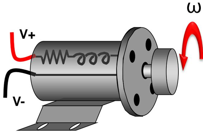
$$V_{in} = K_b \omega + i_m R_m + L_m \frac{di_m}{dt}$$
