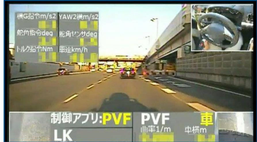
Testing the ACC algorithm using model predictive control on a public road.
