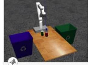
Setup an end-to-end pick and place workflow for a robotic manipulator like the KINOVA® Gen3 and simulate the robot in a physics
