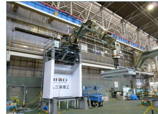
Rendering of Mitsubishi Heavy Industries' seven-meter-long robotic arm capable of withstanding up to 2000 kg of processing reaction force
