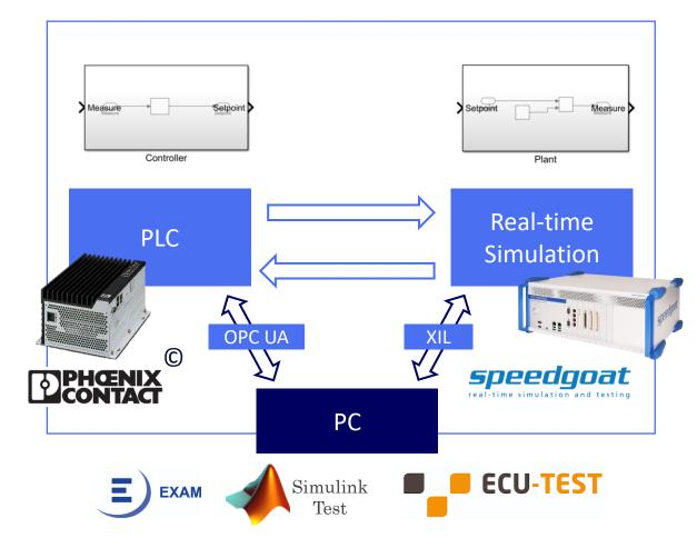
Test physical hardware with a representative model of the plant
