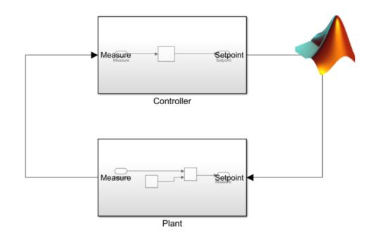
Test closed loop behaviour with a representative model of the plant
