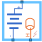
Battery Equivalent Circuit
