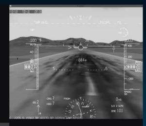
Fixed Pipeline OpenGL implementation in Simulink, Auto-coded using HDL Coder for embedding in an FPGA
