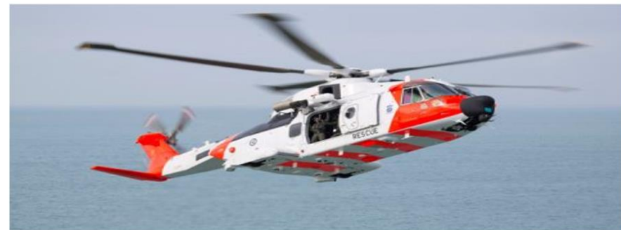
An AW101 long-range helicopter equipped with a Leonardo Osprey 30 active electronically scanned array radar system.
