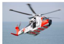
An AW101 long-range helicopter equipped with a Leonardo Osprey 30 active electronically scanned array radar system.
